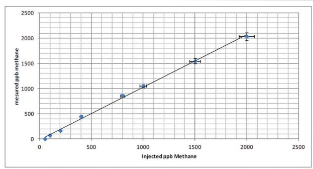
Figure 2. Linearity curve for methane using high amplification
