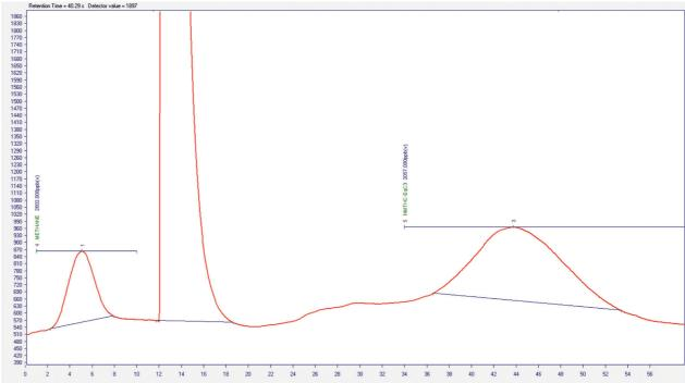
Figure 1. Analysis of a methane / propane cylinder with commutation peak at 13s
