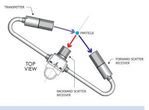
Figure 1: Top view of a Biral present weather sensor showing transmitted and scattered near infrared paths.
