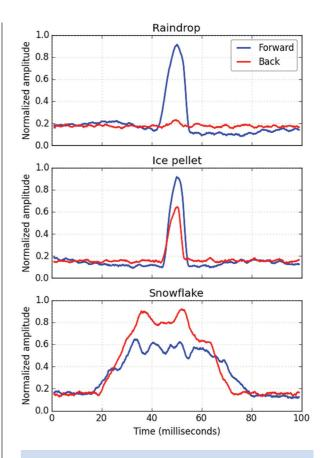
Figure 3: Measured near infrared (850 nm) forward and back scattered amplitudes for different individual hydrometeors as they travelled through the sample volume of a Biral VPF-750 present weather sensor. These measurements were taken as rain (top plot) turned to ice pellets (middle plot) then snow (lower plot) during a thunderstorm over Bristol, UK on 2 March 2016.
