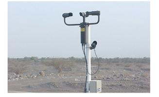
The back scatter receiver is unique to the Biral present weather sensors and provides reliable discrimination between rain and snow. This is demonstrated by reports of excellent snowdetection and discrimination capability from our customers and
