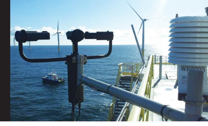
Automatic visibility and present weather sensors normally use the forward scattering of infrared light to estimate visibility and classify precipitation. Sensors produced by Biral emit a cone of modulated near infrared (850 nm) from the transmitter head, which is scattered by particles in the air. The intensity of scattering is not the same in all directions, since this is strongly dependent on the shape, size and composition of the particle.
