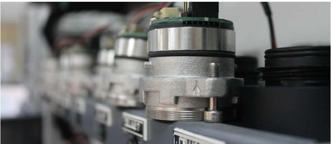
Selection of sensors to be built into gas detection equipment. Copyright Teledyne Gas & Flame Detection
