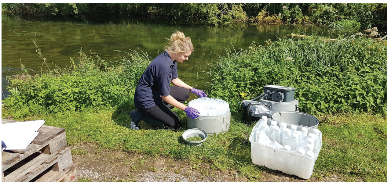
Five automatic samplers collect daily samples from the River Itchen
