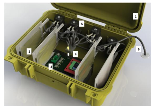
Figure 4 Field deployable platform for the detection of nitrate using chromotropic acid (1) robust and waterproof housing; (2) reagent and standard storage bags; (3) 12 V battery and control board; (4) microfluidic chip and optical detection enclosure; (5) peristaltic pumps containing Viton Tubing; (6) Sample inlet and filter.
