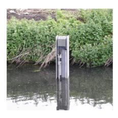
After considering a number of flow measurement options, CEMEX asked Flowline to provide a metering station which would continuously measure the river flows to provide data for use in calibrating a hydraulic model of the Erewash and Attenborough lake system. Another important consideration was that the site was open and accessible to the public and incidents of vandalism had occurred, so any equipment installed had to be as robust as possible, without being too intrusive.
