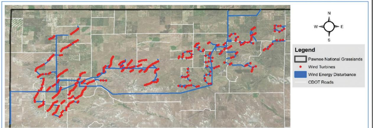
Figure 4: The footprint of wind development in the study area. Red indicates turbine pads, while blue represents access roads and transmission lines.
