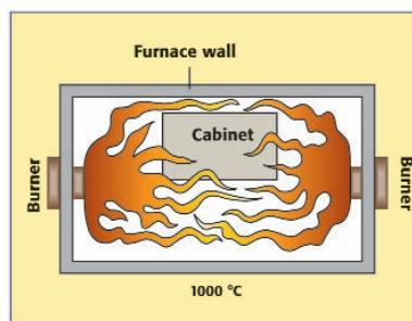
*Furnace test according to BS EN 14470-1*
