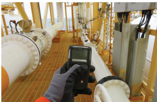
Hand-held portable gas leak detection
