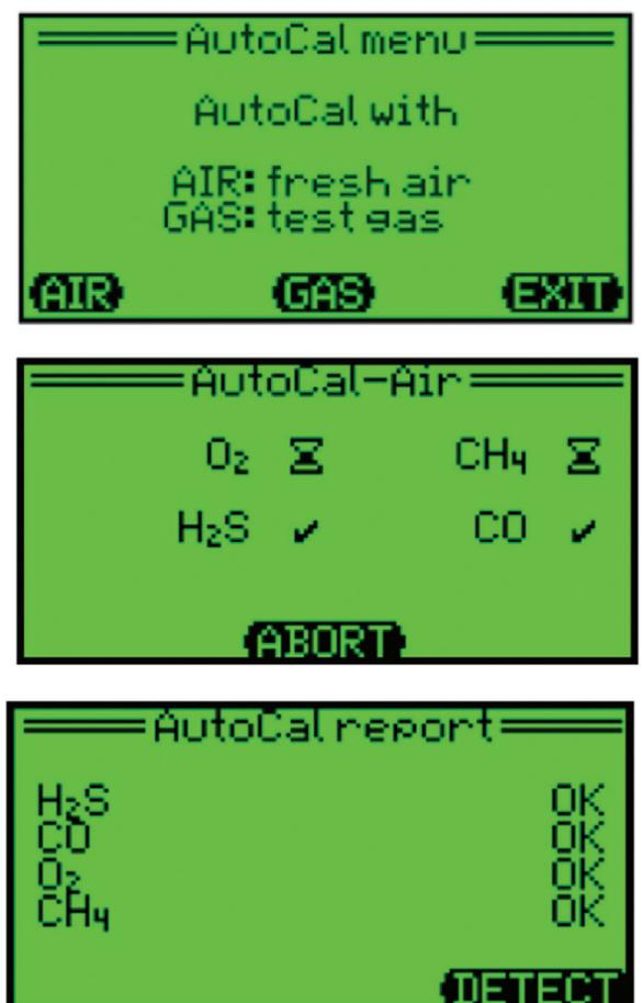
Figure 4: GfG instruments can be automatically fresh air zeroed or calibrated by means of a simple "AutoCal" procedure, (press "Air" to make an automatic fresh air zero adjustment, "Gas" to make a span calibration adjustment, or "Exit" to return to normal operation)
