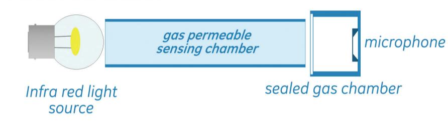
allows gas to permeate through and diffuse in the sensing chamber.
