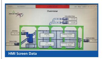
We have provided Advetec with a number of single line gas sampling units (GasVac® Solo) for the monitoring of gases produced within their large scale biodigester machines. With 95% humidity the system is designed to auto drain and purge whilst maintaining a 4-20mA output.
