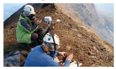
In developing our low-cost, low-power, high-durability instrument based on electrochemical sensors, we highlight the strong potential for electrochemical sensors to contribute to long-term volcano monitoring. The field-deployments demonstrated the capability of electrochemical sensors to endure the harsh, acidic environment of a volcano and to detect a range of gases in the plume-mixture, through newly developed
