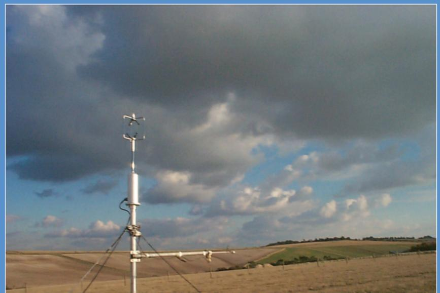
**A Hydra Mark 4 integrated open-path, dual gas eddy correlation system monitoring water vapour and carbon dioxide flux on the Berkshire Downs**
