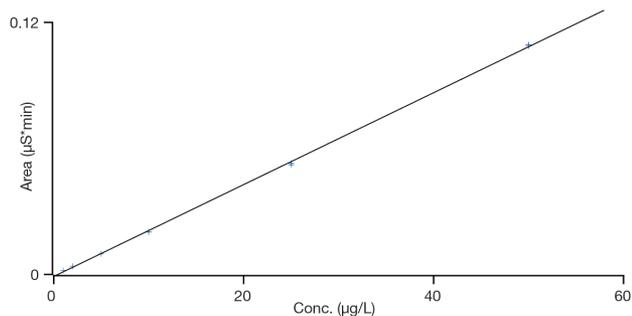
Figure 3. Perchlorate calibration curve
