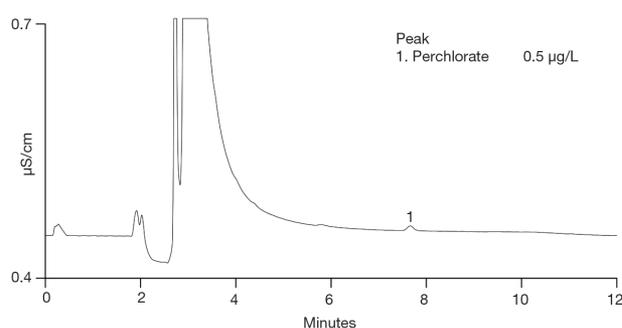
Figure 6. Determination of 0.5 µg/L perchlorate in DI water
