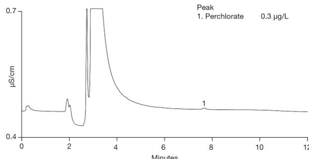
Figure 5. Determination of 0.3 µg/L perchlorate in DI water
