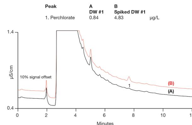
Figure 8. Overlay of chromatograms of (A) DW #1 and (B) spiked DW #1
