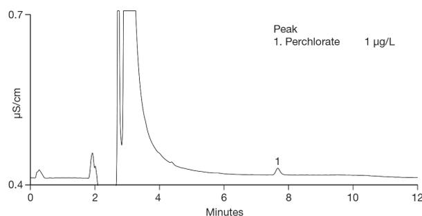
Figure 4. Determination of 1 µg/L perchlorate in DI water
