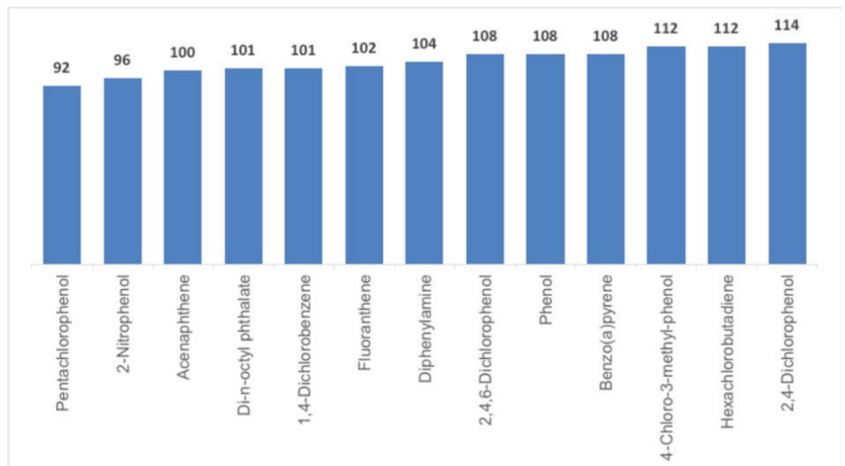
Figure 4. Analyte recovery (%) after repeated sludge injections (n=50)
