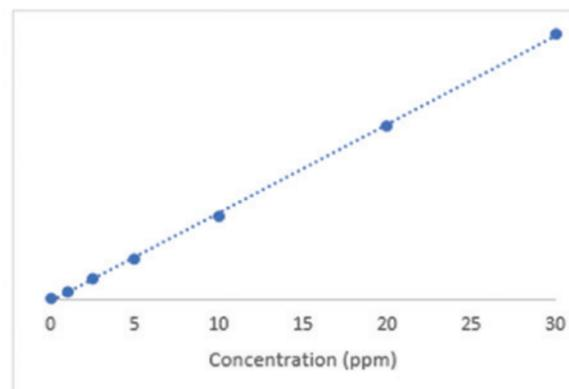
Figure 3. Calibration curve of hexachlorocyclopentadiene, a system performance check
