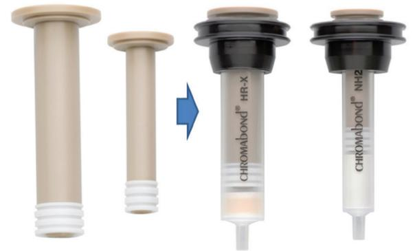
The CVUA-MEL uses for clean-up the MACHERY-NAGEL CHROMABOND columns, which are particularly suitable for the fast and effective sample clean-up in the robotic device. In order to minimize dead volumes in the columns and to increase the flow rates, LCTech has developed special plungers that are inserted into the columns.
