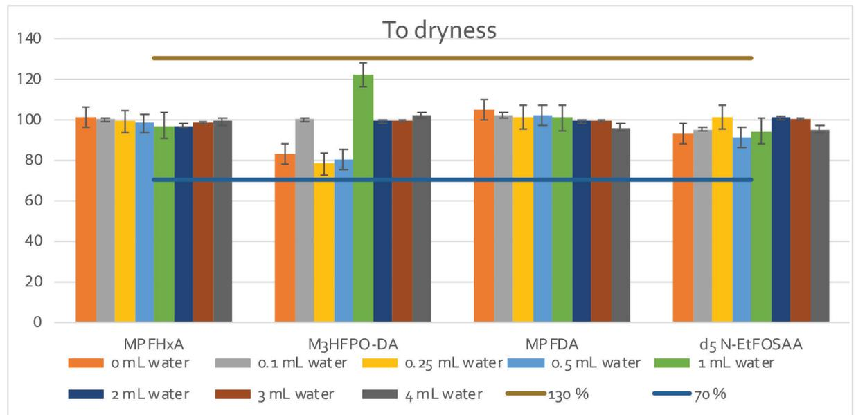
Fig. 3: Comparison of recoveries with regards to residual water
