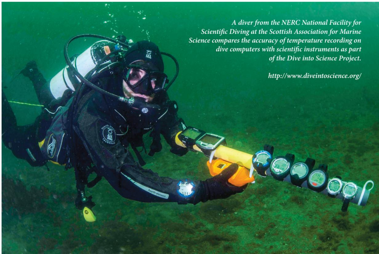
*A diver from the NERC National Facility for Scientific Diving at the Scottish Association for Marine Science compares the accuracy of temperature recording on dive computers with scientific instruments as part of the Dive into Science Project.*
