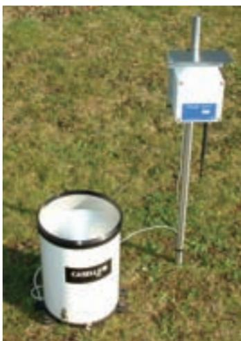
programmes. The recommended density of stations for weather and rainfall is 20km, so that they will need to be powered in ways other than by mains electricity such as solar power. These stations will also have to have the capability to transmit records via mobile data services such as GSM or GPRS in real time in order to offer early warning of extreme weather or rainfall events.
