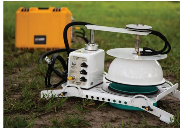
Soil gas exchange chambers are designed to minimize disturbance to the soil environment.
