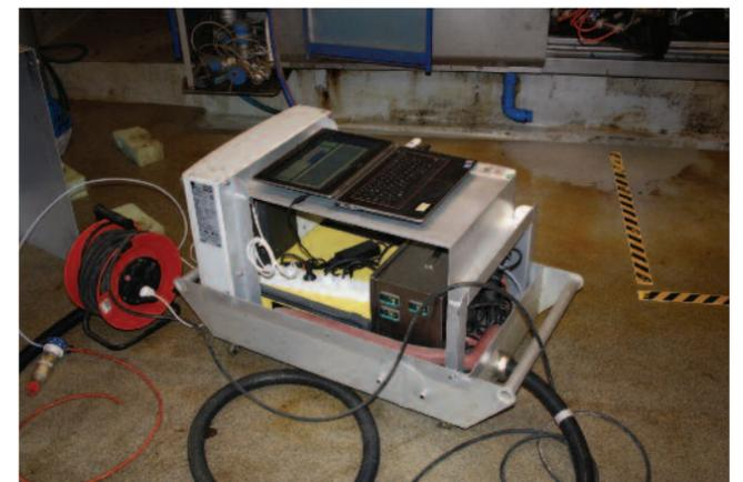
Gaset's Danish Distributor C.K Environment A/S constructed a special cradle to protect the analyser and computer from the 'special conditions' inside a milking parlour
