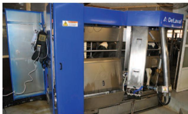
Initially a portable Gaset FTIR was used to capture cow breath for analysis
