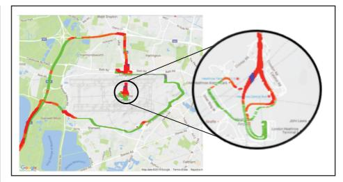
Figure 2: Total NOx levels from Duvas gas test at Heathrow airport, Aug 2016
