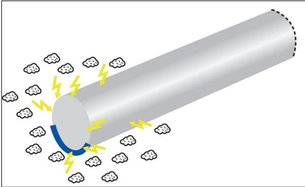
Pic 3. Triboelectric Measuring Principle
