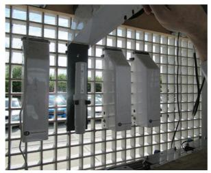
The EDT is a single gas monitor and users can select from a range of gases at the time of ordering. These include  $NO_2$ ,  $NO_2 + O_3$ ,  $SO_2$ ,  $H_2S$ , NO,  $NH_3$  and CO, with relative humidity and ambient temperature also being recorded for every measurement. Typical applications include monitoring urban air quality, checking livestock welfare, and recording waste water treatment and other odour nuisances.
