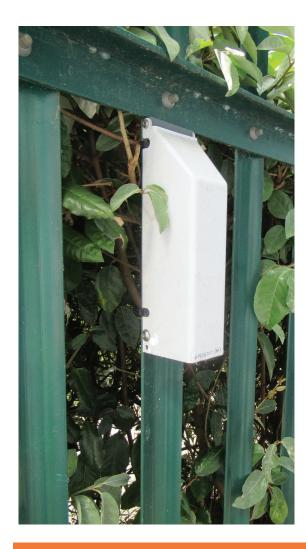
The Alphasense EDT is ideal for this application and was supplied pre-calibrated and set to record concentrations every two minutes. Mounted in the protective bracket, the EDT was quickly and easily mounted on a fence in an ideal location, running on internal batteries and logging data to an internal SD-card.
